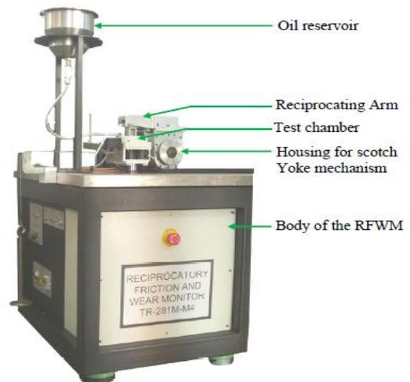
**Fig. 1.** Photographic view of the Reciprocatory Friction and Wear Monitor.
