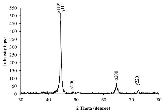
**Fig. 2.** X-ray diffraction pattern of the sample subjected to CHT.
