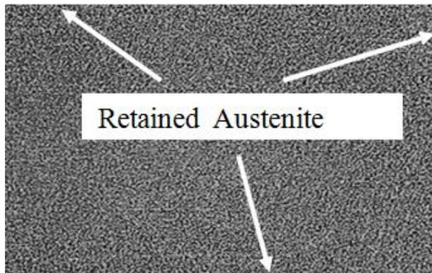
**Fig. 6.** Microstructure of the Sample Subjected to CHT.
