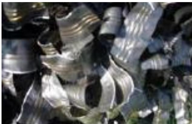
Fig.2. Polyethylene tape used by Nacheva *et al.* [23] as packing material.
