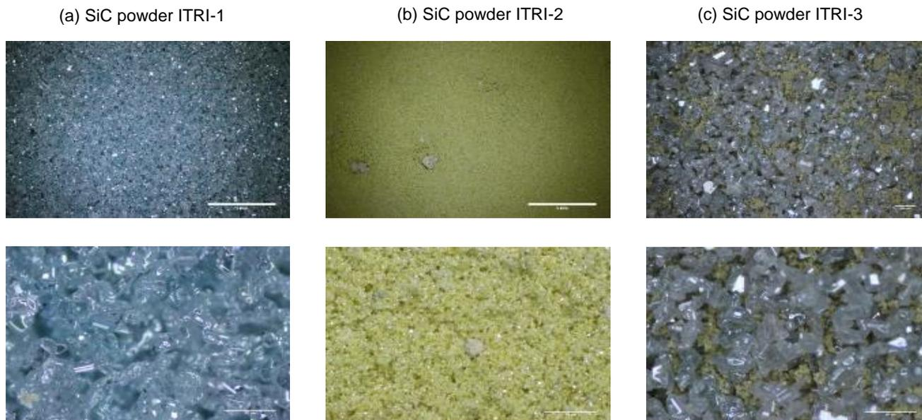
**Fig. 1.** Optical microscopy images of the three SiC powder sources ITRI-1, ITRI-2 and ITRI-3.
