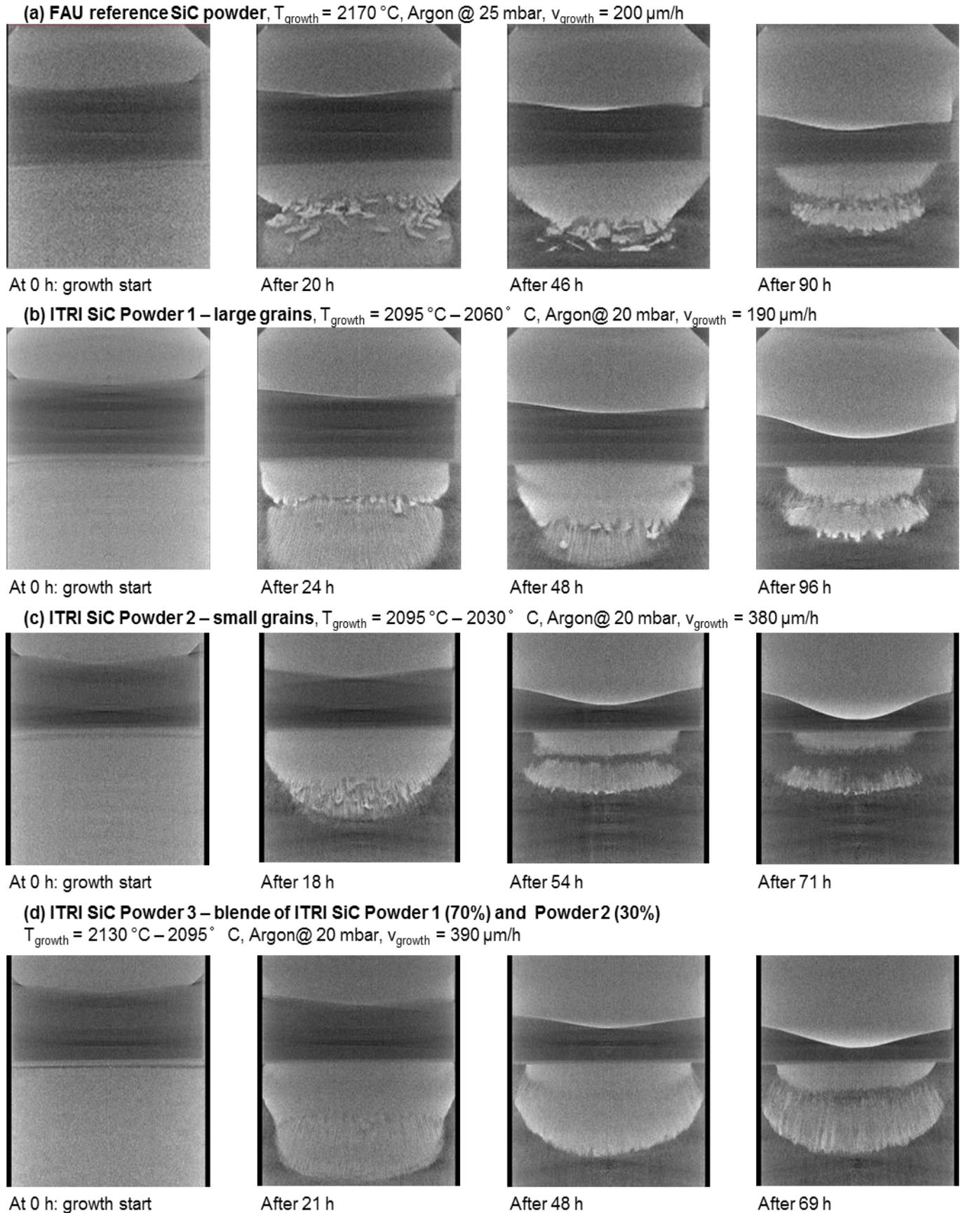
**Figure 2.** Evolution of the SiC source material and SiC powder source using in-situ computed tomography X-ray visualization of the growth process. The 2D projection images are extracted from the 3D data sets. (a) Reference growth run using the FAU reference SiC powder. (b, c, d) SiC powder optimization study using the SiC powders ITRI-1, ITRI-2 and ITRI-3.
