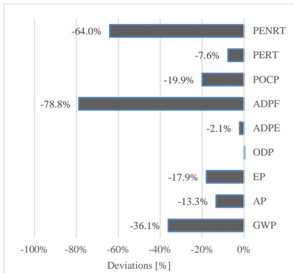
**Fig. 4.** Deviations in % between initial LCA (1:4 allocation ratio, no energy reduction) and LCA based on the “ethanol internal used”-scenario and a 35 % energy reduction assumption.
