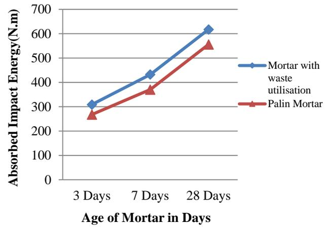
**Fig. 6.** Relation between absorbed impact energy with age of concrete.
