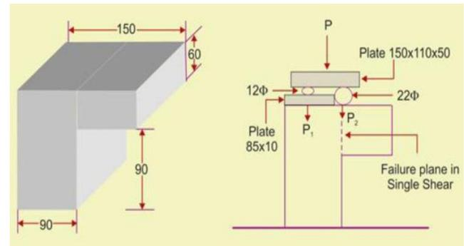
**Fig. 1.** L shape specimen for shear strength test.
