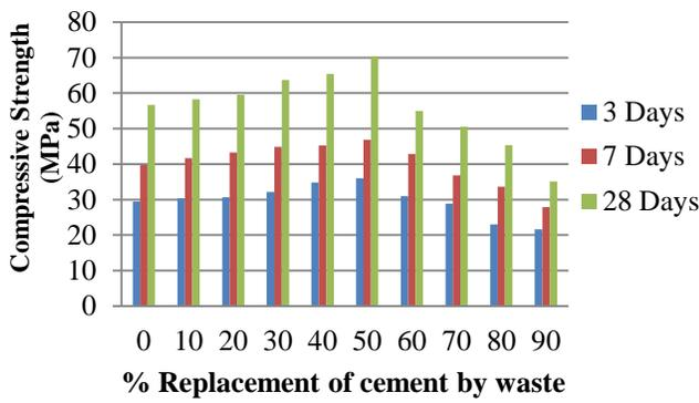
**Fig. 3.** Relation of compressive strength of mortar with percentage of waste powder as cement replacement.
