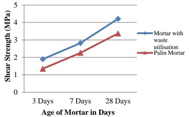
**Fig. 5.** Relation between shear strength and age of mortar.
