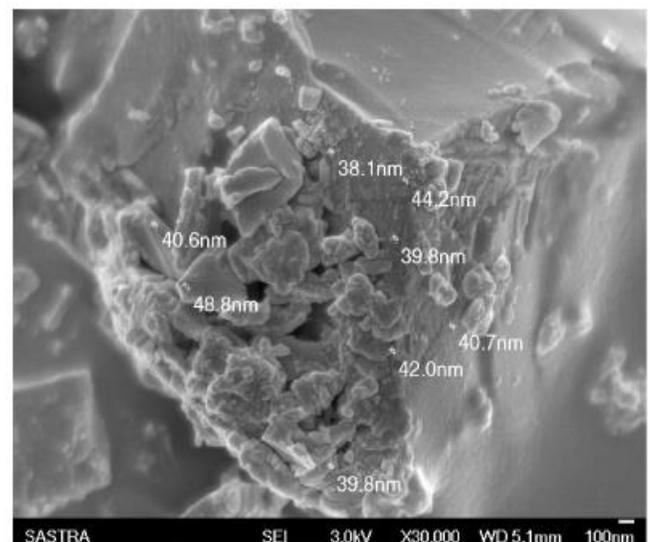
**Fig. 2.** SEM image of concrete modified with nano slag [7]
