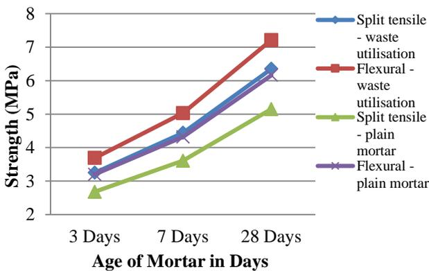
**Fig. 4.** Relation of split tensile Strengths and Flexural Strength with age of mortar.
