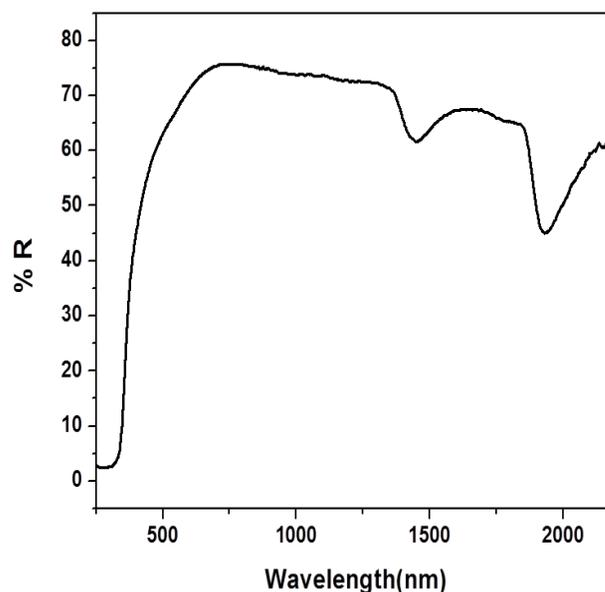
Fig. 2. The Diffuse reflectance spectra of TiO<sub>2</sub>/CdS/BaZnS
