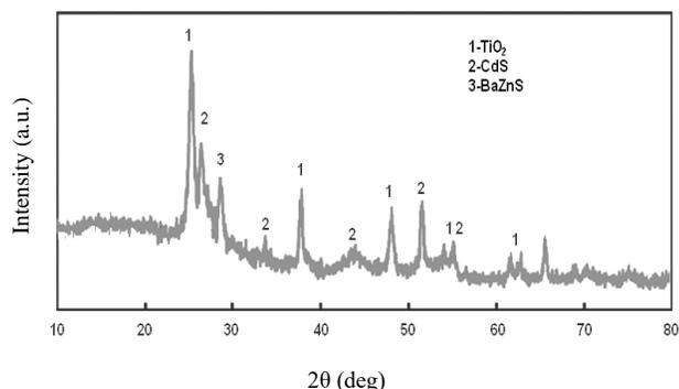
**Fig. 3.** XRD pattern of photoanode FTO/TiO<sub>2</sub>/CdS/BaZnS
