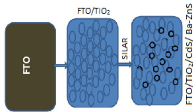
Fig. 1. Schematic presentation of fabrication process of photoanode.
