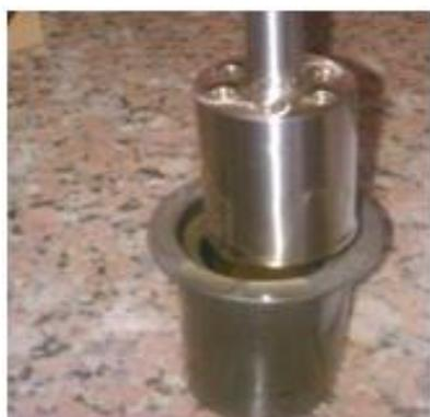
Fig. 2. Concentric cylindrical geometry of Rheometer.
