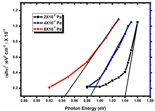
**Fig. 2.** (αhν)<sup>2</sup> Vs hν of Ag<sub>2</sub>O films at various O<sub>2</sub> pressure.
