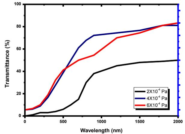
**Fig. 1.** Spectra of optical transmittance at various O<sub>2</sub> pressure.
