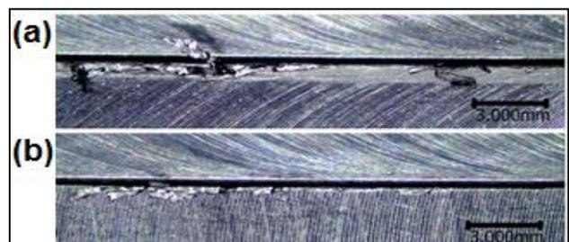
Fig. 5. The variation of burr forms according to MQL flow rate in MQL milling with uncoated WC cutting tool a) 20 ml/h b) 40 ml/h.
