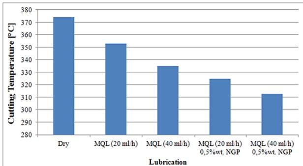
Fig. 2. The variation of cutting temperature with lubrication for uncoated WC cutting tool.
