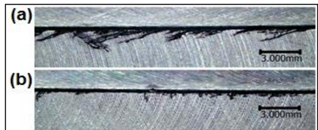
Fig. 4. Burr forms a) uncoated WC and b) TiN coated WC.
