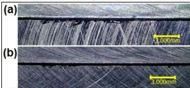
**Fig. 6.** The effect of nanofluid on burr forms for TiN coated WC cutting tool at MQL flow rate of 40 ml/h a) vegetable cutting fluid b) vegetable cutting fluid reinforced by 0,5%wt. nano graphene.
