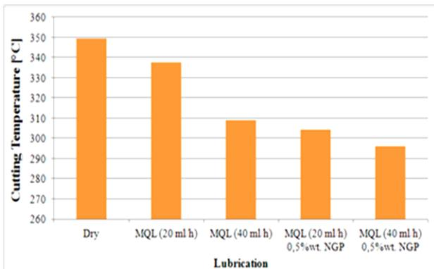
Fig. 3. The variation of cutting temperature with lubrication for TiN coated WC cutting tool.
