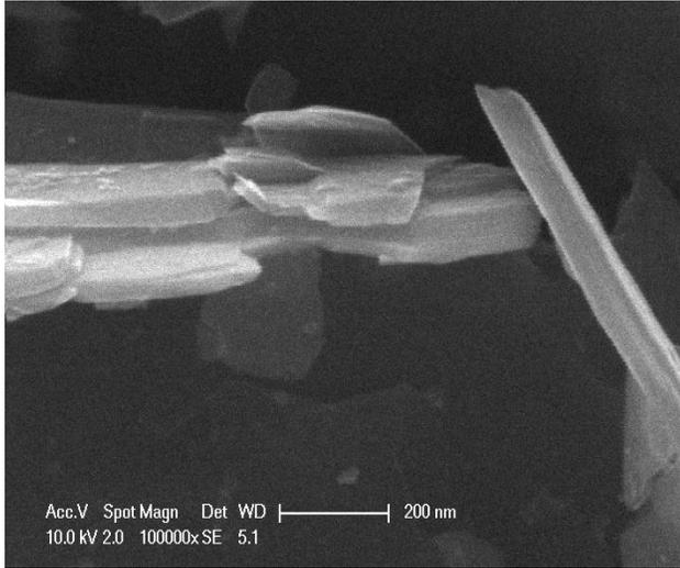
Fig. 1. SEM images of nano graphene
