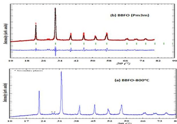
Fig. 1. (a) XRD profile pattern of Bi<sub>0.8</sub>Ba<sub>0.2</sub>FeO<sub>3</sub> ceramic sintered at 800°C (b) profile fitting using FULLPROF program.
