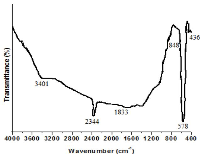
Fig.2: FTIR spectra of Bi<sub>0.8</sub>Ba<sub>0.2</sub>FeO<sub>3</sub> ceramic sintered at 800°C.
