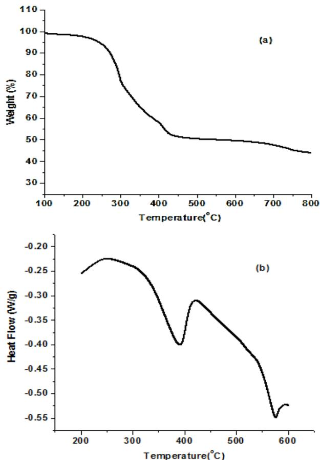
**Fig.3:**(a) TG curve of dried gel  $\text{Bi}_{0.8}\text{Ba}_{0.2}\text{FeO}_3$  ceramic (b) DSC curve of  $\text{Bi}_{0.8}\text{Ba}_{0.2}\text{FeO}_3$  ceramic.
