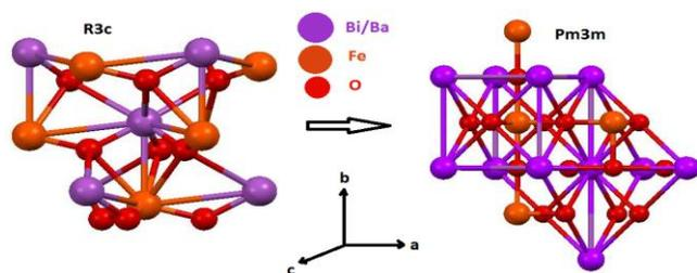
Fig. Structural Transition in Barium substituted BiFeO<sub>3</sub>(BFO).
