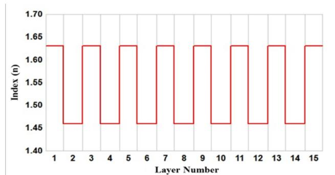
Fig. 2. Quarter wave design of 15 alternating layers of Al<sub>2</sub>O<sub>3</sub> and SiO<sub>2</sub>.
