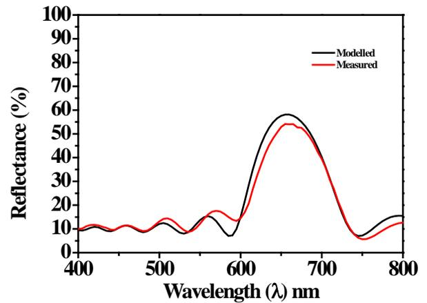
Fig. 5. Reflectance Vs wavelength spectra of Dichroic beam splitter.
