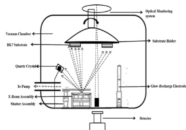
Fig. 3. Schematic of E-beam evaporation plant.
