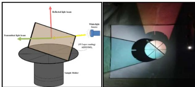
Fig. 4. (a) A schematic of Beam Splitter (b) An experimental setup used for testing of Beam Splitter.
