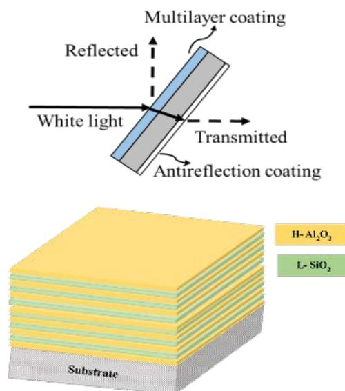
Fig. 1. Schematic showing the transmission and reflection of light through interfaces in dichroic beam splitter.
