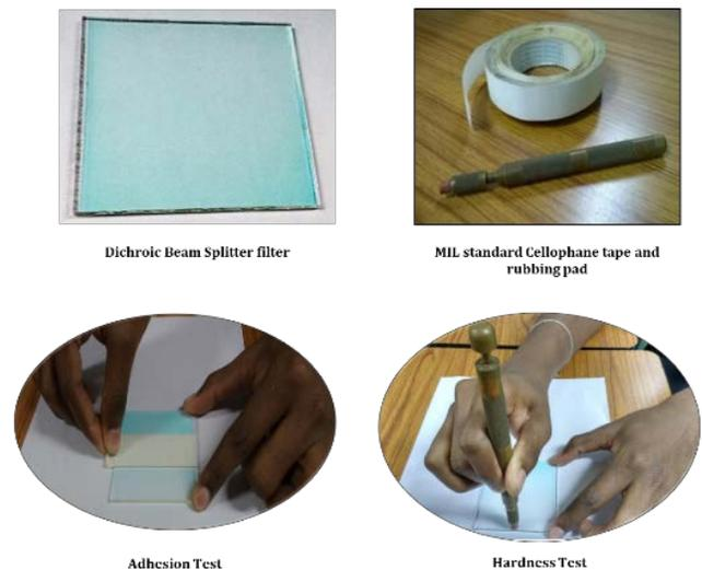
Fig. 6. Film quality test for dichroic beam splitter.
