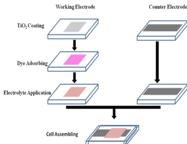
Fig.2: Preparation of cell components and assembling of final DSSC
