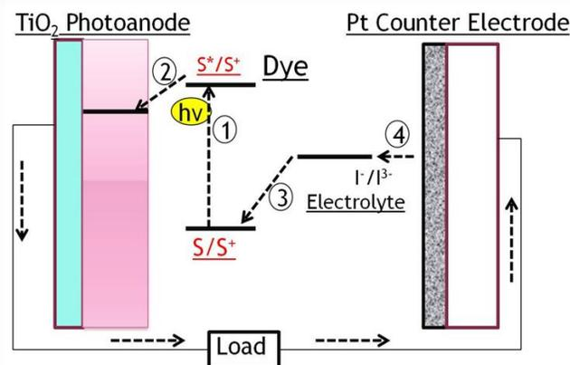
Fig. 1. A schematic diagram representing working principle of DSSCs.
