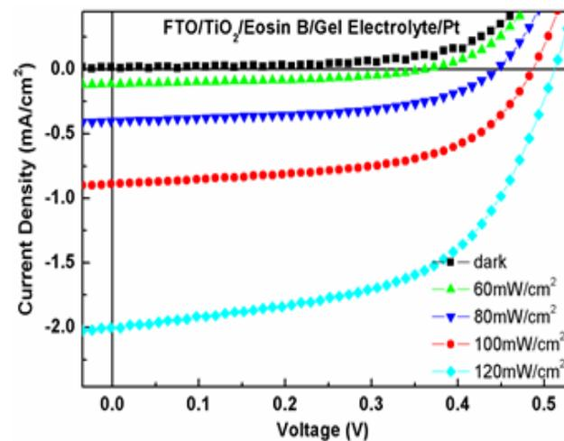
Fig. 4. (a) Current density versus voltage characteristics.
