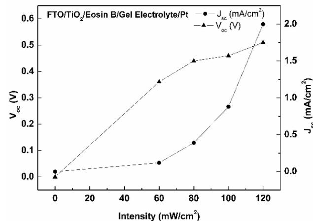
Fig. 5. (b) J<sub>sc</sub> and V<sub>oc</sub> values as a function of illumination intensity.
