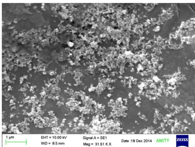
Fig. 3: SEM image of sintered nc-TiO<sub>2</sub> coated glass surface.
