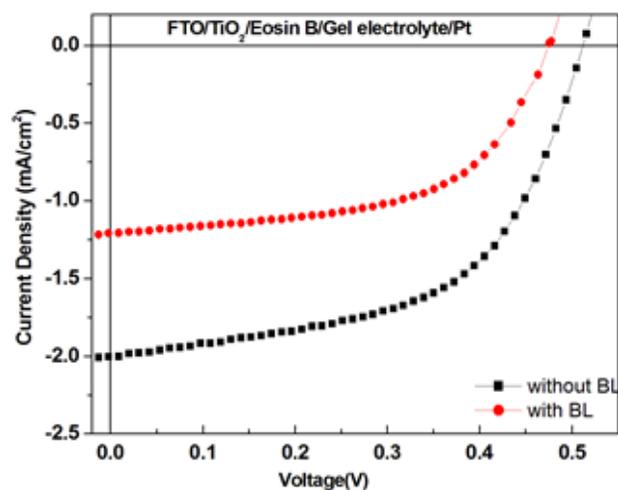
**Fig. 5.** Current density-voltage characteristics of the devices with and without blocking layer at  $120 \text{ mW/cm}^2$ .
