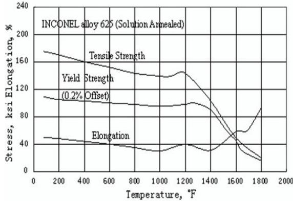
Fig. 5. Mechanical properties of Inconel 625.
