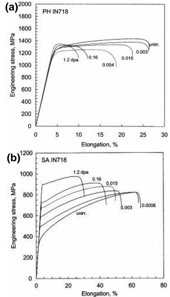
**Fig. 4.** Change in mechanical properties of Inconel 718 with irradiation. (a) Stress-strain curve of Inconel 718 (hardened) at various doses and (b) stress-strain curve of Inconel 718 (solution annealed) at various doses.
