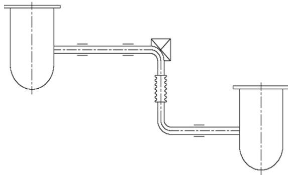
Fig. 2. Use of bellows in piping system to absorb thermal expansions.
