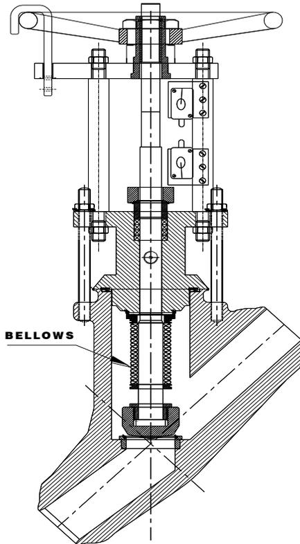
Fig. 1. Schematic of typical bellows sealed sodium valve.
