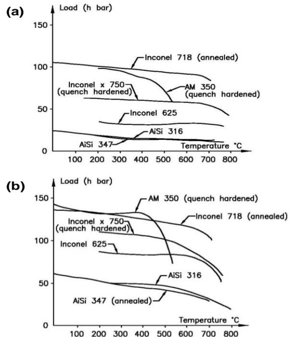
Fig. 6. (a) YS of the candidate materials of bellows and (b) UTS of the candidate materials of bellows
