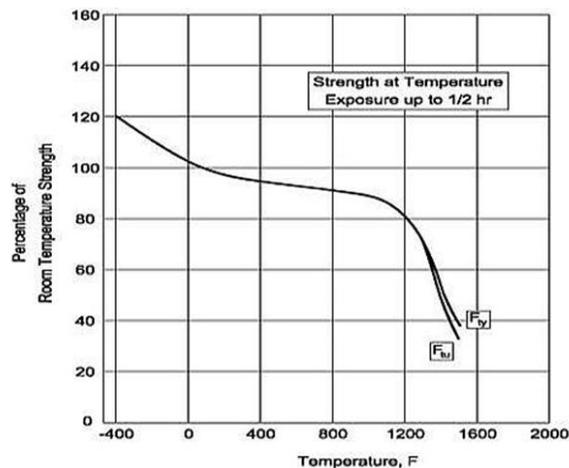
**Fig. 3.** High temperature strength of Inconel 718.
