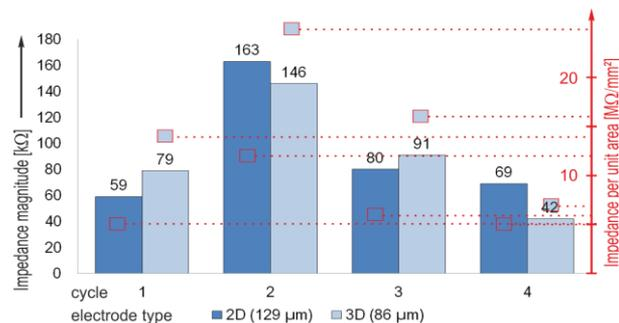
**Fig. 5.** Median of the electrode impedance magnitude and impedance per unit area, measured at 1 kHz for the type c MEA, thick film gold. One cycle encompasses the laminin coating after the described protocol, after each cycle the MEAs are cleaned with tergazyme. After repeated coating the measurement was repeated.
