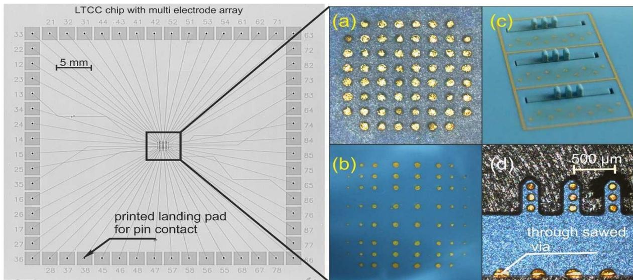
**Fig. 2.** X-ray image of the LTCC chip with 2D electrode layout; the respective electrode area is varied in three types:
