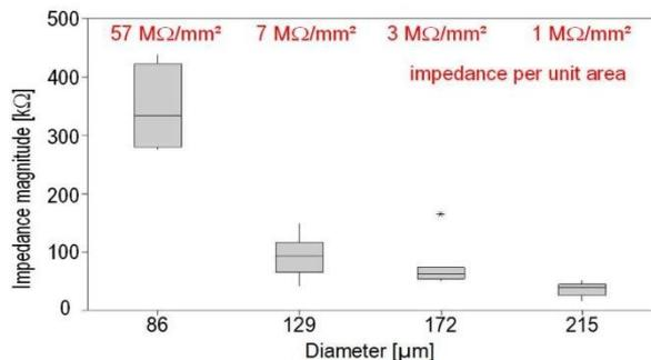
**Fig. 4.** Impedance magnitude dependency on electrode diameter (thick film gold electrodes, nominal frequency 1 kHz, chip type b).
