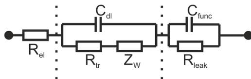
**Fig. 8.** Equivalent circuit of a functionalized electrode.  $R_{el}$ -resistance of the electrolyte;  $C_{dl}$ -double layer capacitance;  $R_{tr}$ - charge transfer resistance;  $Z_W$  - Warburg impedance;  $C_{func}$  - capacitance of the functional layer;  $R_{leak}$ - leak resistance of the functional layer.
