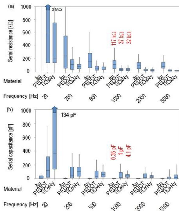
**Fig. 6.** SEC elements plotted over frequency, comparison of measurements on 86  $\mu\text{m}$  electrodes; data base: Au = pure thick film gold – type c; PEDOT = PEDOT:PSS coated thick film gold – type a and TiO<sub>2</sub>N<sub>y</sub> = sputter coated thick film gold – type a; a) serial resistance; b) serial capacitance.
