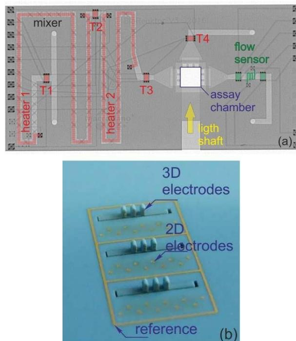
**Fig. 1.** Ceramic bio-reactor. (a) X-ray image, visualizing integrated mixer, temperature control and flow monitoring; (b) ceramic contact board, perpendicularly mounted through slots of the ceramic base plate.
