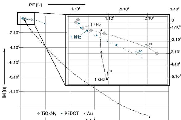
**Fig. 7.** Nyquist plot of median values for thick film gold electrodes, pure and coated with PEDOT:PSS and  $\text{TiO}_x\text{N}_y$ . The data points for PEDOT:PSS and  $\text{TiO}_x\text{N}_y$  represent the medians of all measurements on chip of type a. The data points for Au represent the medians of all measurements on  $86 \mu\text{m}$  electrodes on chip of type c.
