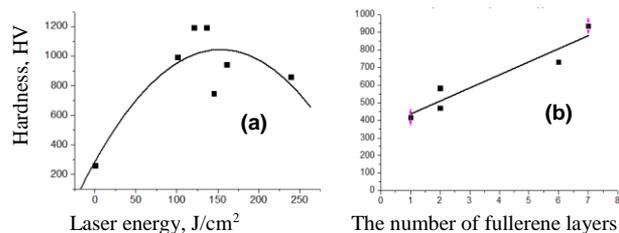
Fig. 2. (a) Dependence of the microhardness of the steel surface - coated with 7 fullerene layers on the laser energy; (b) Dependence of the microhardness of the steel surface on the number of fullerene  $\text{C}_{60}$  layers measured at a laser irradiation energy of  $163 \text{ J/cm}^2$ .
