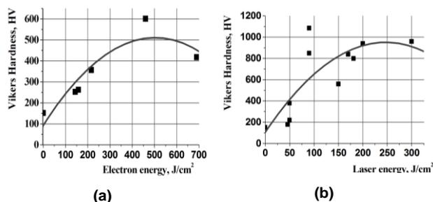
Fig. 1. Dependence of the microhardness of the steel surface with nanocarbon coating on e-beam (a) and laser (b) irradiation energy.
