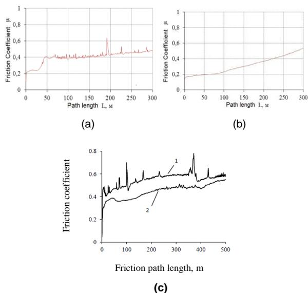
**Fig. 4.** Results of tribology tests of steel samples: (a) Nanocarbon coverage without laser treatment; (b) Nanocarbon coverage with laser treatment; (c) fullerene C<sub>60</sub> (3 layers) coverage with (1) and without (2) laser treatment.
