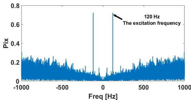
**Fig. 9.** The frequency response of 1ms magnetic pulses at a repetition rate of 120Hz.
