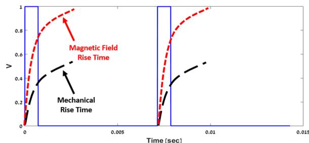
**Fig. 7.** Short pulses generation with respect to the mechanical rise time.
