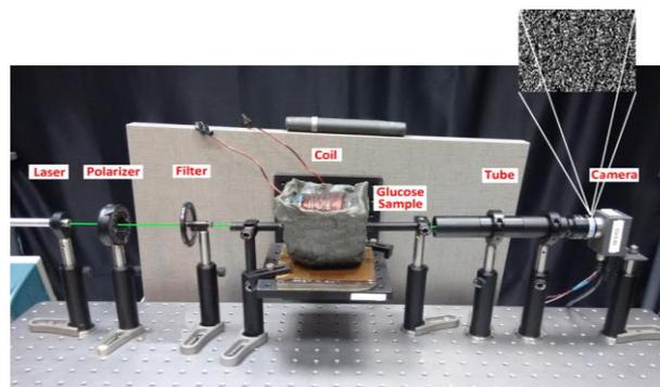
**Fig. 8.** The remote configuration for the magneto optic effect.
