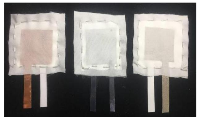
Fig. 2 Three PVDF sensor prototypes produced by different material electrodes (A -adhesive copper foil tape, B - ITO thin plate, C - adhesive conductive cloth).
