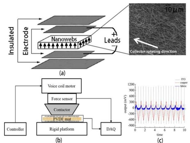
Fig. 1. Packaging structure of the PVDF nanofibers web as sensor prototype.
