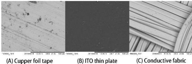
**Fig. 5.** SEM image of three kinds of electrodes
