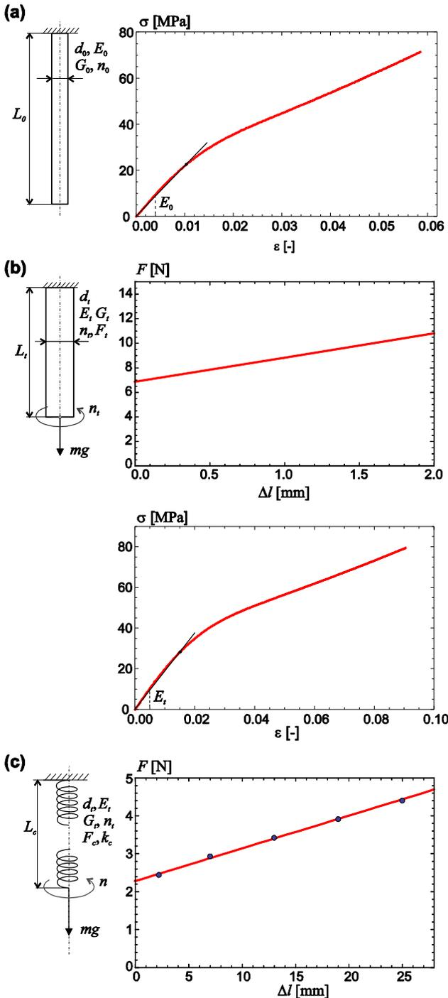
Fig. 2. (a) To measurement of the material properties of the fishing line, (b) to measurement of the material properties and prestress force of the twisted the fishing line, (c) to measurement of the spring constant and prestressing force of the partially unwound spring.
