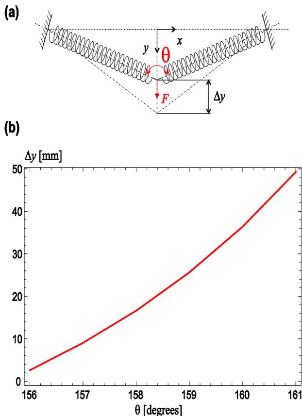
**Fig. 6.** (a) The Von Mises actuator made of fishing line springs, (b) dependence of the vertical displacement  $\Delta y$  on the angle  $\theta$ .
