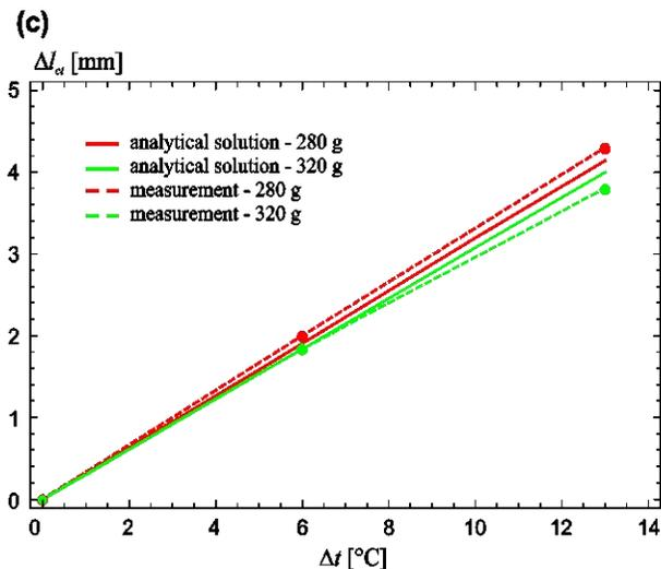
Fig. 5. The measurement and calculation of the thermoelastic elongation of the spring:(a) device for the measurement, (b) the simplified mechanical model for analytical solution, (c) comparison of the analytical solution and the measurement.
