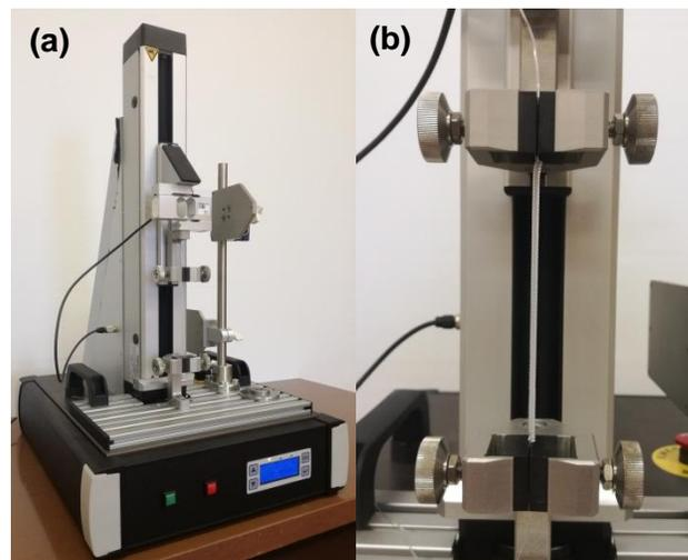
**Fig. 1.** (a) Testing machine for measuring mechanical properties (b) a sample of the coiled spring.
