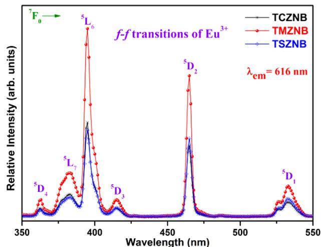
**Fig. 1.** Excitation spectra of 1 mol %  $\text{Eu}^{3+}$ -doped TRZNB glasses.
