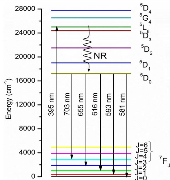
**Fig. 3.** Energy level diagram showing emission transitions of 1.0 mol %  $\text{Eu}^{3+}$ -doped TRZNB glasses.
