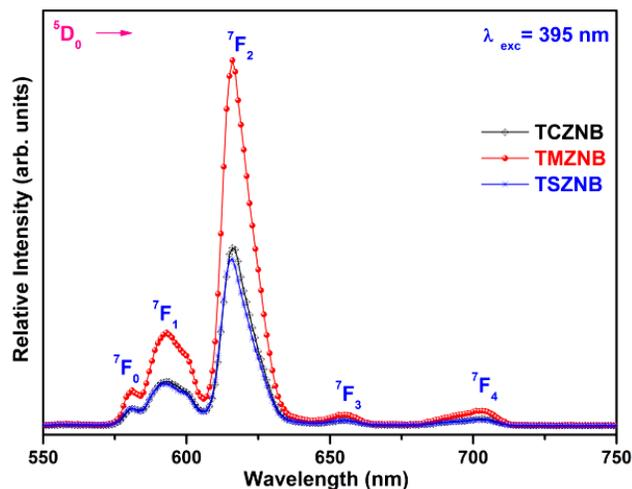
**Fig. 2.** Emission spectra of 1 mol %  $\text{Eu}^{3+}$ -doped TRZNB glasses.
