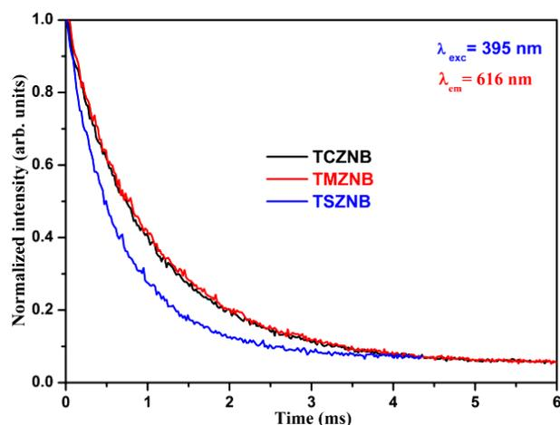
**Fig. 4.** The decay profiles of  ${}^5D_0$  level of 1.0 mol %  $\text{Eu}^{3+}$ -doped TRZNB glasses.
