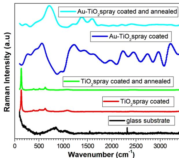
**Fig. 2.** Raman spectra of the glass substrate; TiO<sub>2</sub> spray coated; TiO<sub>2</sub> spray coated and annealed; Au-TiO<sub>2</sub> spray coated; Au-TiO<sub>2</sub> spray coated and annealed samples.
