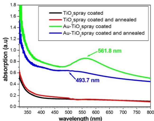
**Fig. 3.** Ultra violet-visible (UV-Vis) absorption spectra of the TiO<sub>2</sub> spray coated; TiO<sub>2</sub> spray coated and annealed; Au-TiO<sub>2</sub> spray coated; Au-TiO<sub>2</sub> spray coated and annealed samples.
