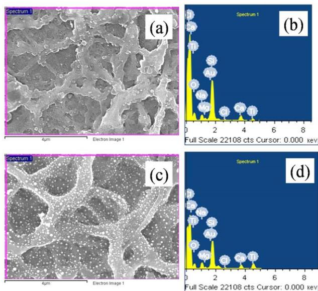
**Fig. 6.** (a) FESEM micrograph area selected for EDX pattern of Au- $\text{TiO}_2$  spray coated film; (b) EDX pattern of Au- $\text{TiO}_2$  spray coated film; (c) FESEM micrograph area selected for EDX pattern of Au- $\text{TiO}_2$  spray coated annealed film; (d) EDX pattern of Au- $\text{TiO}_2$  spray coated annealed film.
