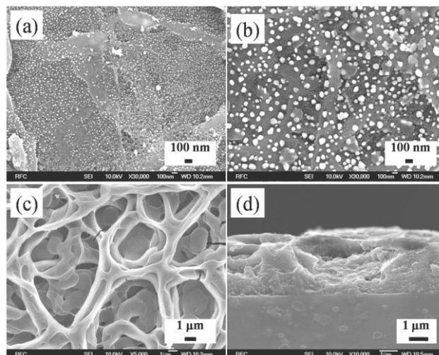
**Fig. 5.** Field emission scanning electron microscopy (FESEM) of (a) Au- $\text{TiO}_2$  spray coated at the 100 nm scale, (b) Au- $\text{TiO}_2$  spray coated and annealed samples at the 100 nm scale, (c)  $\text{TiO}_2$  spray coated at  $400^\circ\text{C}$  at the 1  $\mu\text{m}$  scale and (d) cross-sectional micrographs of  $\text{TiO}_2$  spray coated at  $400^\circ\text{C}$  at the 1  $\mu\text{m}$  scale.
