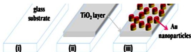
**Fig. 1.** Schematic of thin film grown by spray pyrolysis method for Au-TiO<sub>2</sub> film deposition.
