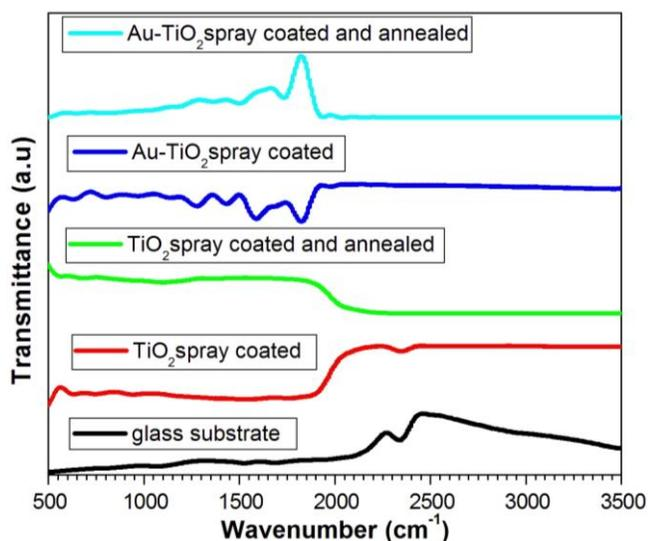
**Fig. 4.** FTIR spectra of the glass substrate;  $\text{TiO}_2$  spray coated;  $\text{TiO}_2$  spray coated and annealed; Au- $\text{TiO}_2$  spray coated; Au- $\text{TiO}_2$  spray coated and annealed samples.
