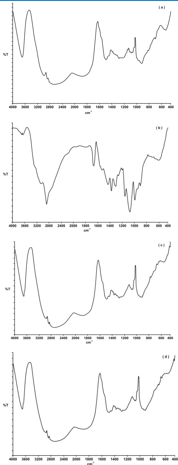
Fig. 3. FTIR spectrum of the (a) graphite, (b) chitosan, (c) graphite doped chitosan composite before lead (II) adsorption and (d) graphite doped chitosan composite after lead (II) adsorption.
