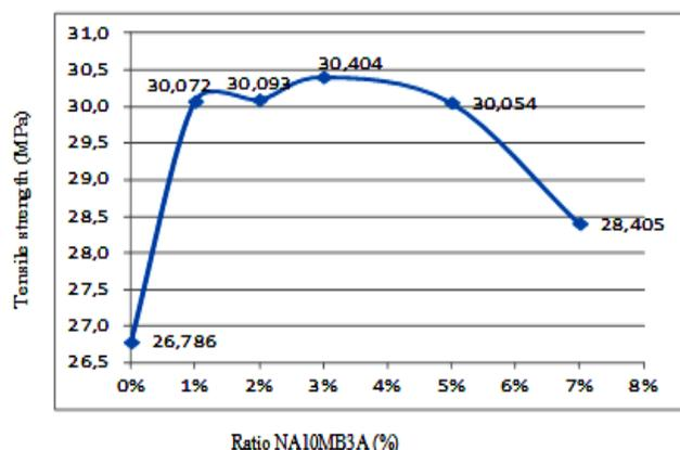
**Fig. 6.** Schematic diagram of the relationship between the ratio of Na10MB3A (%) and the tensile strength of PP.
