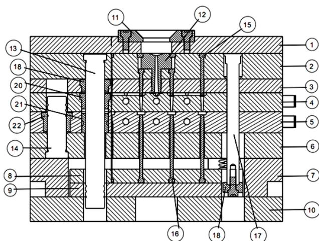
Fig. 1. Injection mold used to produce experimental specimens.
