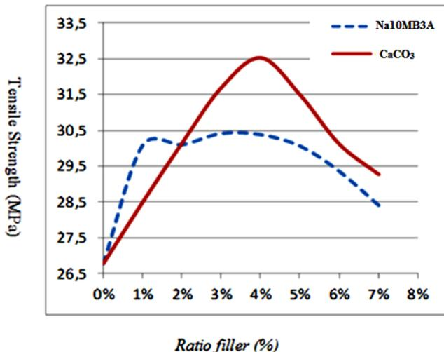
Fig. 10. Comparison of two curves in Figs. 6 & 8 in the range from 0% to 7%.
