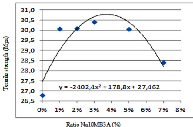
**Fig. 7.** The quadratic polynomial interpolation curve presents the relationship between the tensile strength PP (MPa) and the ratio of added Na10MB3A (%).
