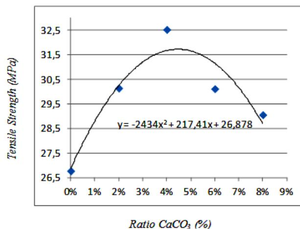
**Fig. 9.** The quadratic polynomial interpolation curve gives the relationship between the tensile strength of PP (MPa) and the ratio of added  $\text{CaCO}_3$  (%).
