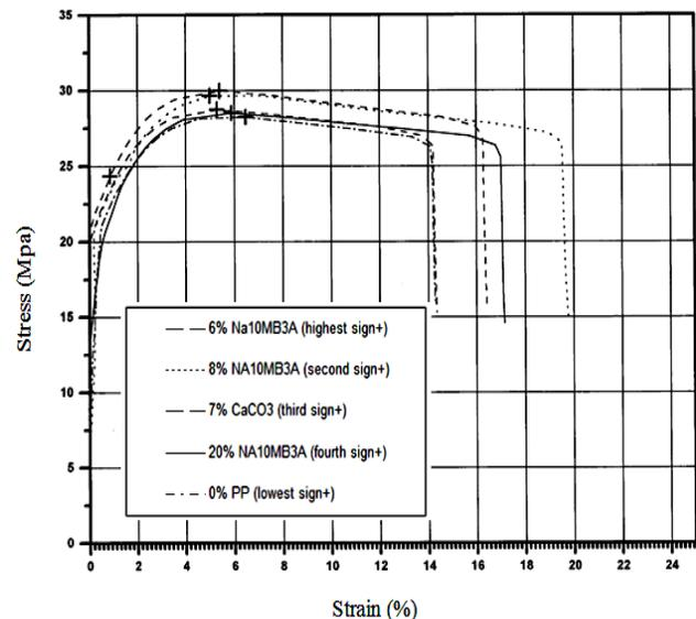
**Fig. 5.** Strain-stress curve diagram for PP filler-reinforced specimens.
