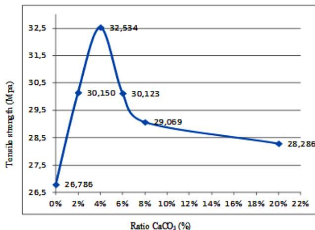
**Fig. 8.** Schematic diagram showing the relationship between the ratio of added  $\text{CaCO}_3$  (%) and the tensile strength of PP (MPa).
