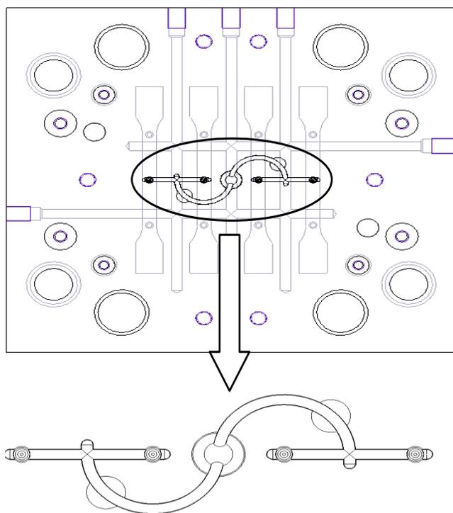
Fig. 2. General structure of channel and product arrangement.
