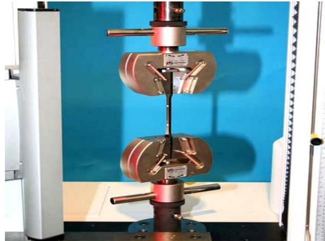
**Fig. 4.** Tensile test machine Instron 5566-CN2081.
