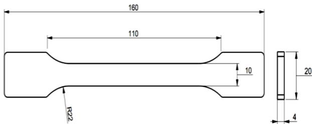
**Fig. 3.** Polypropylene specimen.
