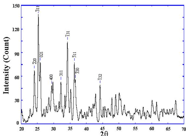
Fig. 1. X-ray diffraction pattern of SrAl<sub>4</sub>O<sub>7</sub>:Dy phosphor matched with JCPDS data file no. 25-1208.
