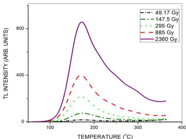
Fig. 3. TL Glow curve of SrAl<sub>4</sub>O<sub>7</sub>:Dy(15%) irradiated with different doses of  $\gamma$  radiation.
