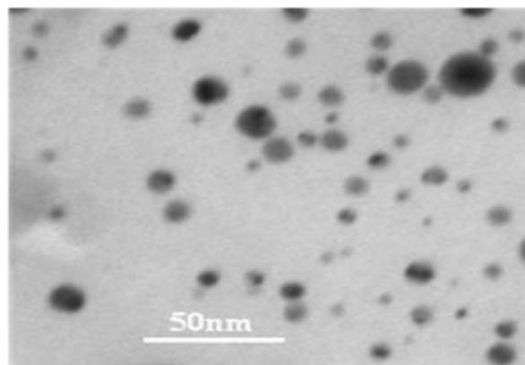
**Fig. 4.** TEM image of Ag nanoparticles in PVP prepared by  $\gamma$ -irradiation.
