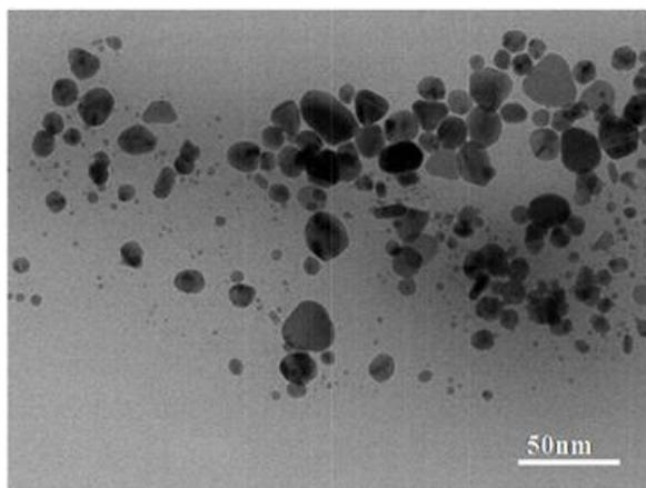
**Fig. 2.** TEM image of Ag nanoparticles in PVP prepared by X-ray irradiation.
