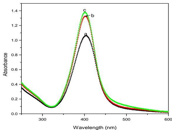
**Fig. 3.** Absorption spectra of aqueous Ag nanoparticles in PVP prepared by  $\gamma$ -irradiation for different absorption dose: (a) 1kGy, (b) 1.3kGy, (c) 1.6kGy;  $[Ag^+] = 2 \times 10^{-4} \text{ mol. dm}^{-3}$ ,  $[PVP] = 0.5\%$ ,  $[Isopropanol] = 2 \times 10^{-1} \text{ mol. dm}^{-3}$ , dose rate =  $4.0 \text{ kGy.h}^{-1}$ ; The solution was two times diluted before taking spectra.
