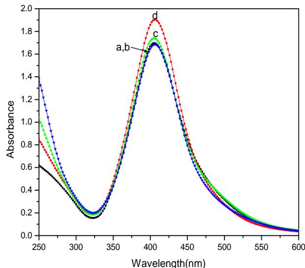
**Fig. 8.** Absorption spectra of aqueous Ag nanoparticles in PVP prepared by X-ray irradiation for different PVP concentration: (a) 0.1%, (b) 0.5%, (c) 1%, (d) 2% (w/v); [ $\text{Ag}^+$ ]=  $2 \times 10^{-4}$  mol.  $\text{dm}^{-3}$ , [Isopropanol]=  $2 \times 10^{-1}$  mol.  $\text{dm}^{-3}$ , dose= 2.0kGy, dose rate=  $113.7 \text{ kGy} \cdot \text{h}^{-1}$
