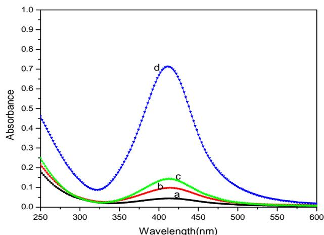
**Fig. 1.** Absorption spectra of aqueous Ag nanoparticles in PVP prepared by X-ray irradiation for different irradiation time: (a) 12s, (b) 23sec, (c) 41s, (d) 63s;  $[Ag^+] = 2\times 10^{-4}$  mol. dm<sup>-3</sup>,  $[PVP] = 0.5\%$ ,  $[Isopropanol] = 2\times 10^{-1}$  mol. dm<sup>-3</sup>, dose rate= 113.7kGy.h<sup>-1</sup>.
