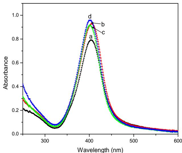
**Fig. 9.** Absorption spectra of aqueous Ag nanoparticles in PVP prepared by  $\gamma$ -irradiation for different PVP concentration: (a) 0.1%, (b) 0.5%, (c) 1%, (d) 2% (w/v); [ $\text{Ag}^+$ ]=  $2 \times 10^{-4}$  mol.  $\text{dm}^{-3}$ , [Isopropanol]=  $2 \times 10^{-1}$  mol.  $\text{dm}^{-3}$ , dose= 2.0kGy, dose rate=  $4.0 \text{ kGy} \cdot \text{h}^{-1}$ ; The solution was three times diluted before taking spectra.
