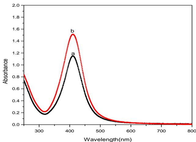
**Fig. 11.** Absorption spectra of aqueous Ag nanoparticles in PVP prepared by EB- irradiation for different absorption dose rate: (a) 2.4kGy/s, (b) 1.2kGy/s;  $[Ag^+] = 2 \times 10^{-4} \text{ mol. dm}^{-3}$ ,  $[PVP] = 0.5\%$ ,  $[Isopropanol] = 2 \times 10^{-1} \text{ mol. dm}^{-3}$ , dose rate= 2.0kGy.
