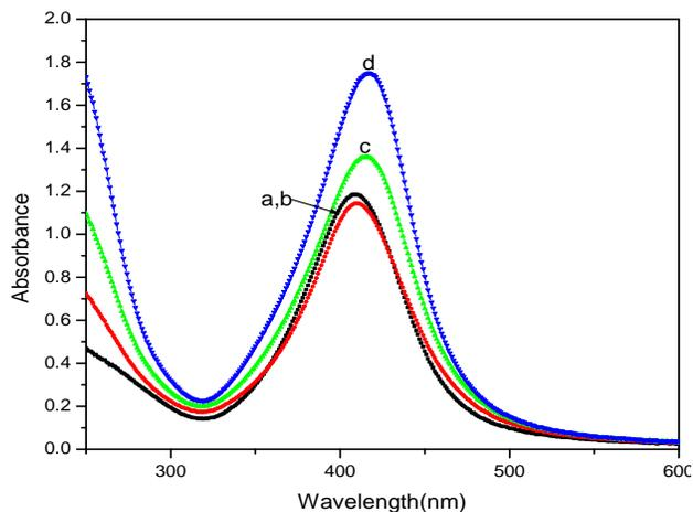
**Fig. 10.** Absorption spectra of aqueous Ag nanoparticles in PVP prepared by EB- irradiation for different PVP concentration: (a) 0.1%, (b) 0.5%, (c) 1%, (d) 2% (w/v);  $[Ag^+] = 2 \times 10^{-4} \text{ mol. dm}^{-3}$ ,  $[Isopropanol] = 2 \times 10^{-1} \text{ mol. dm}^{-3}$ , dose= 2.0kGy, dose rate= 2.4kGy/s; The solution was two times diluted before taking spectra.
