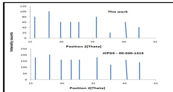
**Fig. 1.** XRD pattern of  $\text{Sr}_2\text{V}_2\text{O}_7 : \text{Eu}^{3+}$  phosphor.
