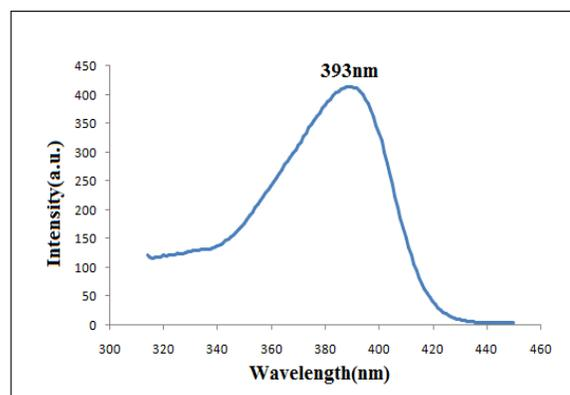
**Fig. 2.** Excitation spectra of  $\text{Sr}_2\text{V}_2\text{O}_7 : \text{Eu}^{3+}$  phosphor.
