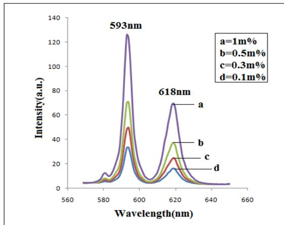
Fig. 3. Emission spectrum of  $\text{Sr}_2\text{V}_2\text{O}_7:\text{Eu}^{3+}$  phosphor.
