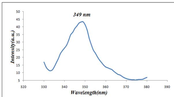
Fig.4 Excitation spectra of  $\text{Sr}_2\text{V}_2\text{O}_7:\text{Dy}^{3+}$  phosphor.
