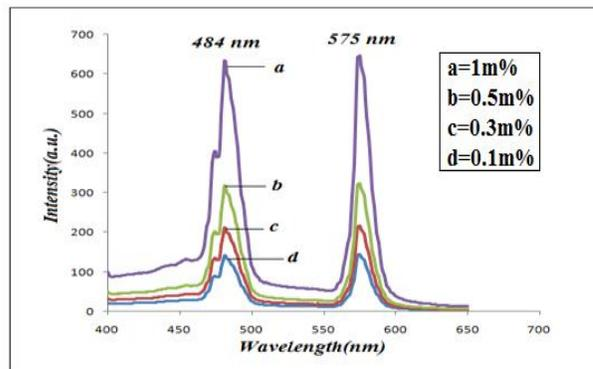
Fig. 5. Emission spectrum of  $\text{Sr}_2\text{V}_2\text{O}_7:\text{Dy}^{3+}$  phosphor.
