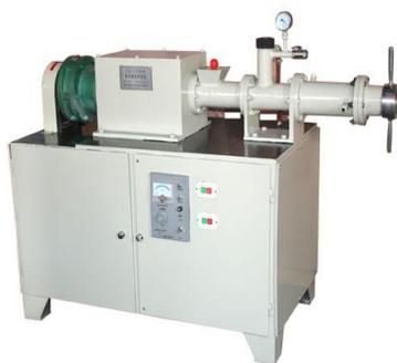
Fig. 2. Photograph of vacuum pug mill.
