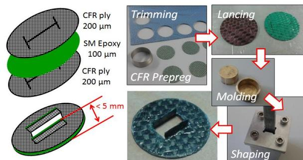
**Fig. 1.** Design and manufacturing of SMPC samples for long-term exposure to Space environment in LEO.
