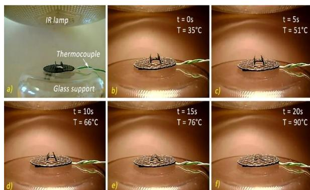
**Fig. 4.** On-Earth Shape recovery of the SMPC samples designed for long-term exposure to Space environment in LEO.
