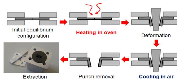
**Fig. 2.** Thermo-mechanical cycle for shape change.
