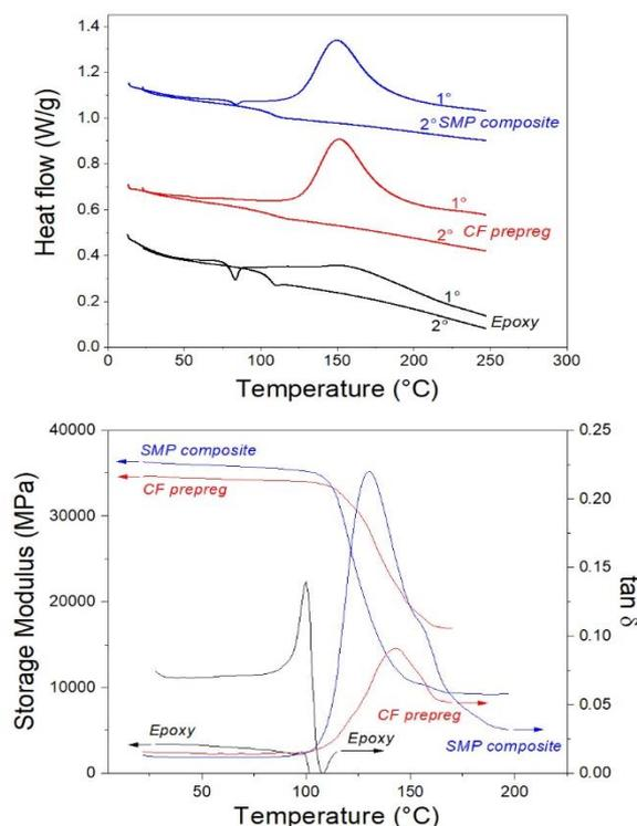
**Fig. 3.** DSC (a) and DMA (b) results from testing CFR laminate, CFR-SMPC laminate and SM epoxy resin.
