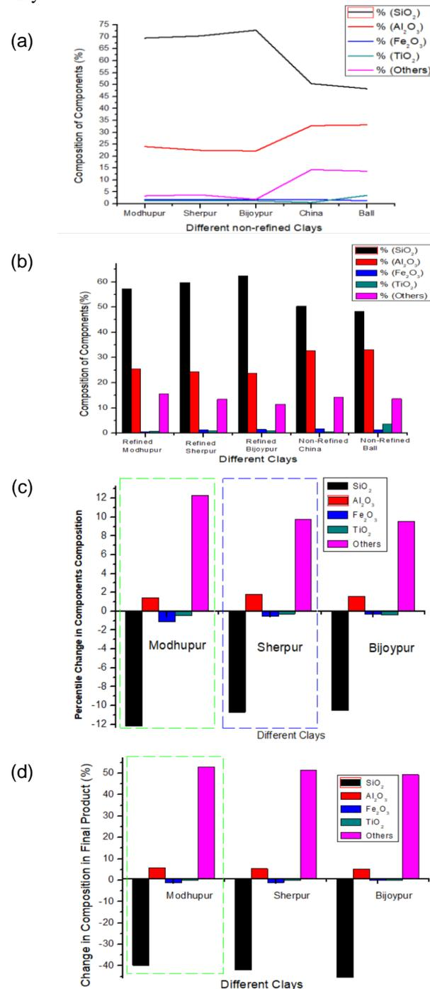
Fig. 5. (a) Non-refined Samples composition, (b) Refined local clay samples in contrast to imported china and ball clay, (c) Percentile point change in new refined local clay samples and (d) Change in composition in refined local clay samples from the non-refined samples.
