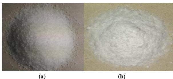
Fig. 2. (a) Sodium silicate deflocculant and (b) Poly-acrylamide flocculant.
