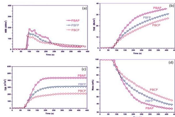
**Fig. 10.** Cone calorimetric plots of synthesized polyphosphazenes (a) HRR (b) THR (c) TSR (d) wt. % residue curves.
