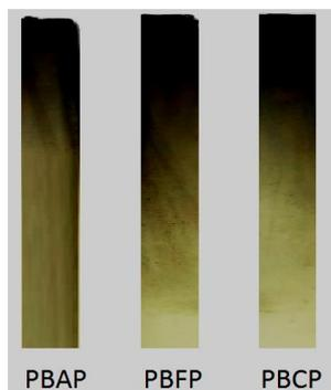
**Fig. 9.** UL-94 vertical burning images of polyphosphazene samples.
