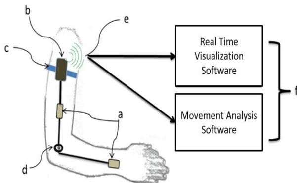
Fig. 1. Inertial and magnetic capture platform.
