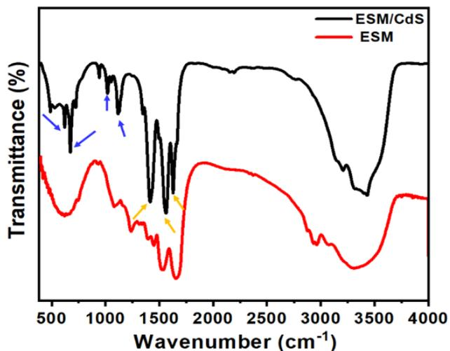
Fig. S3. FT-IR spectra of bare ESM and CdS nanoparticles immobilized ESM samples (yellow arrow represents ESM band; blue arrow represents CdS band).
