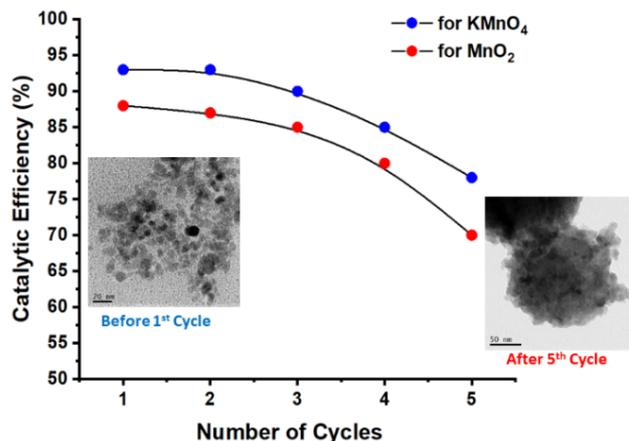
Fig. S4. Plot of catalytic efficiency of CdS nanoparticles as observed up to five cycles (inset: TEM bright-field images of CdS nanoparticles before the 1<sup>st</sup> cycle and after the fifth cycle test, respectively).
