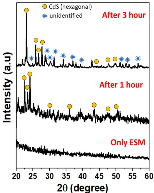
Fig. S2. X-ray diffraction of the pattern of only ESM and ESM derived CdS powder sample after 1 hour and 3 hour of UV irradiation, respectively.
