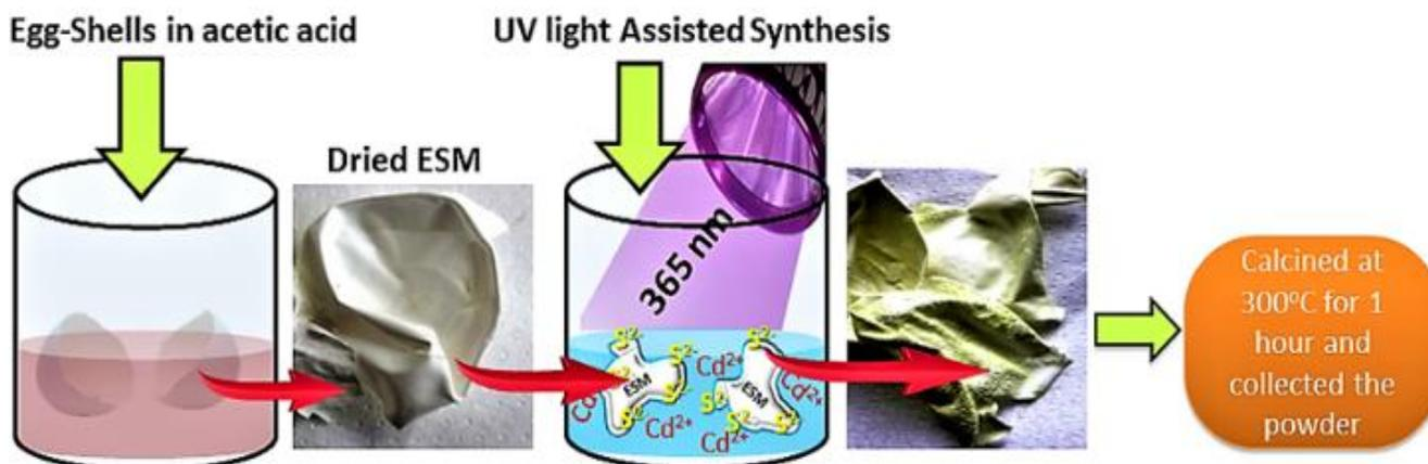
Fig. S1. Schematic representation of ESM assisted CdS nanoparticle synthesis.
